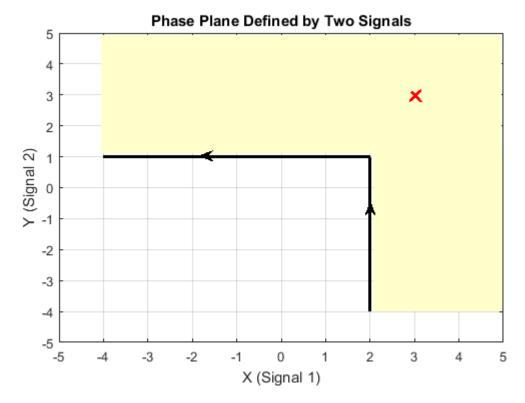
The plot shows that the edges were created in the opposite order. So, even though the requirement type is still '>=', the out-of-bound region, which is always to the right of the edges, is now flipped.
